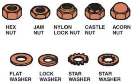
FIGURE 3–16 Various types of nuts (top) and washers (bottom) serve different purposes and all are used to secure bolts or cap screws.
