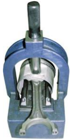
FIGURE 29–36 A press used to remove the connecting rod from the piston.
