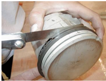
FIGURE 29–42 The side clearance of the piston ring is checked with a feeler gauge.
