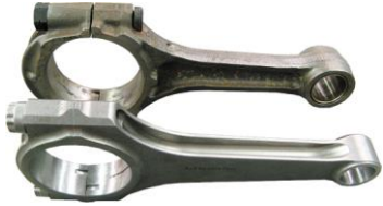
FIGURE 29–28 The I-beam shape is the most common (top connecting rod), but the H-beam shape is common in high-performance and racing engine applications.
