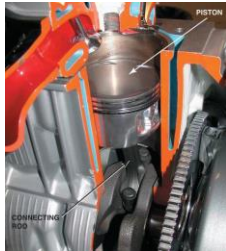
FIGURE 29-1 The piston seals the bottom of the combustion chamber and is attached to a connecting rod.
