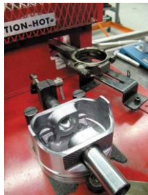
FIGURE 29–41 The small end of the rod is being heated in an electric heater and the piston is positioned properly so the piston pin can be installed as soon as the rod is removed from the heater.
