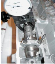
FIGURE 28-44 A dial indicator being used to measure cam lobe height.
