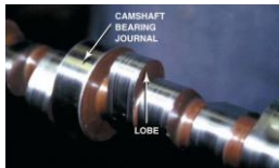
FIGURE 28-1 This high-performance camshaft has a lobe that opens the valve quickly and keeps it open for a long time.
