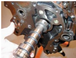
FIGURE 28-3 The camshaft rides on bearings inside the engine block above the crankshaft on a typical cam-in-block engine.
