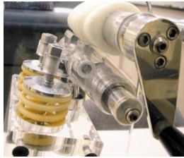
FIGURE 28-53 A plastic mockup of a Honda VTEC system that uses two different camshaft profiles—one for low-speed engine operation and the other for high speed.
