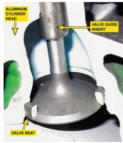
FIGURE 27-35 All aluminum cylinder heads use valve seat inserts. If an integral valve seat (cast-iron head) is worn, it can be replaced with a replacement valve seat by machining a pocket (counterbore) to make a place for the new insert seat.
