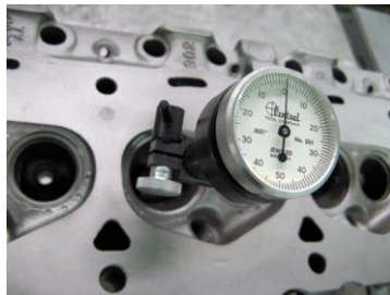
FIGURE 27-31 Checking valve seat concentricity using a dial indicator.
