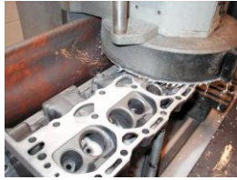
FIGURE 26-22 A cast-iron cylinder head being resurfaced using a surface grinder.
