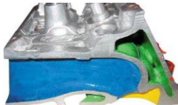
FIGURE 26-14 A cutaway head showing the coolant passages in green.
