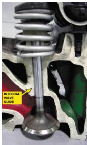
FIGURE 26-26 An integral valve guide is simply a guide that has been drilled into the cast-iron cylinder head.
