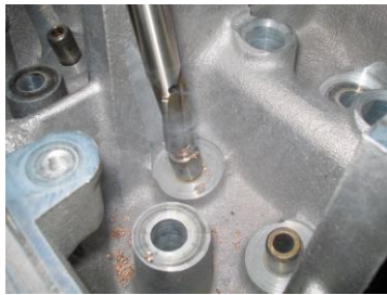
FIGURE 26-35 Trimming the top of the thin-walled insert.
