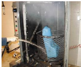
FIGURE 25-5 A pressure jet washer is similar to a large industrial-sized dishwasher. Each part is then rinsed with water to remove chemicals or debris that may remain there while it is still in the tank.
