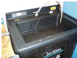
FIGURE 25-6 A microbial cleaning tank uses microbes to clean grease and oil from parts.
