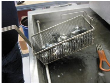
FIGURE 25-8 An ultrasonic cleaner is used to clean fuel injectors.
