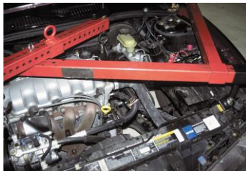
FIGURE 24-4 When removing just the engine from a front-wheel-drive vehicle, the transaxle must be supported. Shown here is a typical fixture that can be used to hold the engine if the transaxle is removed or to hold the transaxle if the engine is removed.
