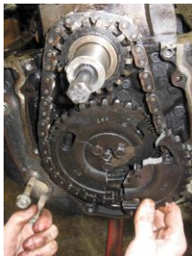
FIGURE 24-13 When the timing chain cover was removed, the broken timing gear explained why this GM 4.3 liter V-6 engine stopped running.
