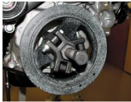
FIGURE 24-12 Puller being used to pull the vibration damper from the crankshaft.
