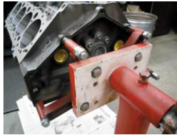
FIGURE 24-6 Always use graded bolts—either grade 5 or 8 bolts—whenever mounting an engine to a stand.
