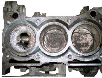
FIGURE 24-8 Sometimes after the cylinder head has been removed, the engine condition is discovered to be so major that the entire engine may need to be replaced rather than overhauled.
