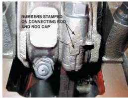
FIGURE 24-9 These connecting rods were numbered from the factory. If they are not, then they should be marked.
