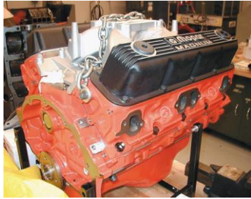
FIGURE 24-2 A crate engine from Chrysler to be used in a restored muscle car. Using a complete new engine costs more than rebuilding an existing engine, but it has a warranty and uses all new parts.
