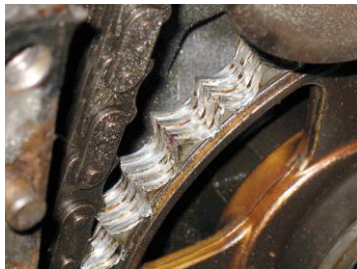
FIGURE 24-1 A worn timing sprocket that resulted in a retarded valve timing and reduced engine performance.
