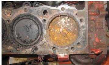
FIGURE 24–15 This small block Chevrolet V-8 had water standing in the cylinders, causing a lot of rust, which was discovered as soon as the head was removed.
