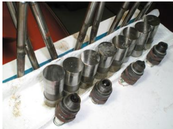
FIGURE 24-7 Keeping the pushrods and the lifters sorted by cylinder, including the spark plugs, is a wise way to proceed when disassembling the cylinder heads.
