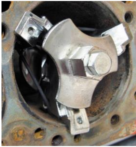
FIGURE 24-11 This ridge is being removed with one type of ridge reamer before the piston assemblies are removed from the engine.
