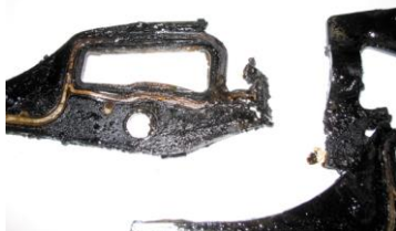
FIGURE 23-3 An intake manifold gasket that failed and allowed coolant to be drawn into the cylinder(s).
