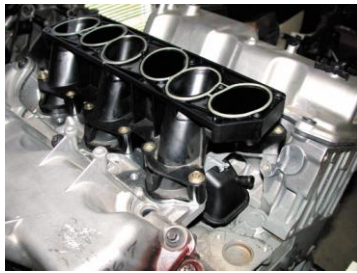
FIGURE 23-4 The lower intake manifold attaches to the cylinder heads.
