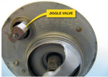
FIGURE 23-1 If the thermostat has a jiggle valve, it should be placed toward the top to allow air to escape. If a thermostat were to become stuck open or open too soon, this can set a diagnostic trouble code P0128 (coolant temperature below thermostat regulating temperature).
