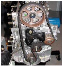
FIGURE 23-7 A single overhead camshaft engine with a timing belt that also rotates the water pump.
