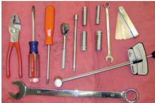
2 The tools necessary to adjust the valves on an engine with adjustable rocker arms include basic hand tools, feeler gauge, and a torque wrench.
