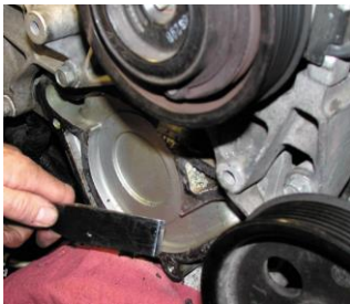
FIGURE 23-2 Use caution if using a steel scraper to remove a gasket from aluminum parts. It is best to use a wood or plastic scraper.
