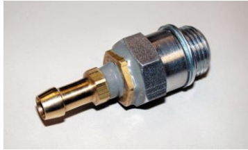
FIGURE 22-28 A technician-made adapter used to test exhaust system back pressure.
