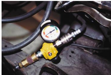
FIGURE 22-14 A typical handheld cylinder leakage tester.
