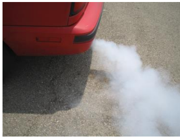
FIGURE 22–2 White steam is usually an indication of a blown (defective) cylinder head gasket that allows engine coolant to flow into the combustion chamber where it is turned to steam.
