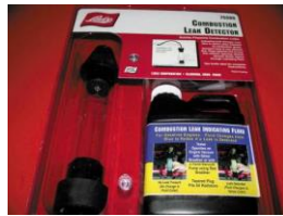
FIGURE 22-29 A tester that uses a blue liquid to check for exhaust gases in the exhaust, which would indicate a head gasket leak problem.
