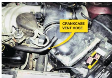
FIGURE 22-1 Blowby gases coming out of the crankcase vent hose. Excessive amounts of combustion gases flow past the piston rings and into the crankcase.
