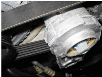
FIGURE 22-6 An accessory belt tensioner. Most tensioners have a mark that indicates normal operating location. If the belt has stretched, this indicator mark will be outside of the normal range. Anything wrong with the belt or tensioner can cause noise.
