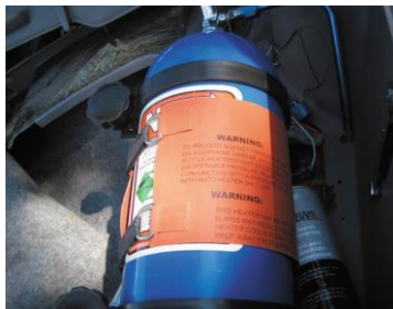
FIGURE 21-17 An electrical heating mat is installed on the bottle of nitrous oxide to increase the pressure of the gas inside.
