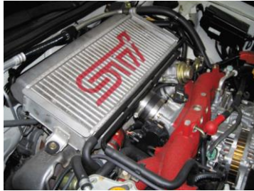
FIGURE 21–12 The unit on top of this Subaru that looks like a radiator is the intercooler, which cools the air after it has been compressed by the turbocharger.
