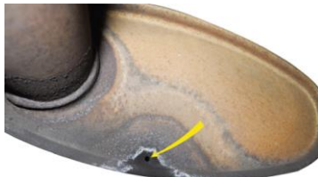
FIGURE 20-21 A hole in the muffler allows condensed water to escape.
