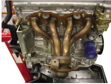
FIGURE 20-16 Many exhaust manifolds are constructed of steel tubing and are free flowing to improve engine performance.
