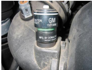
FIGURE 20-4 A typical air filter restriction indicator used on a General Motors truck engine. The indicator turns red when it detects enough restriction to require a filter replacement.
