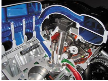
FIGURE 20–11 The air flowing into the engine can be directed through long or short runners for best performance and fuel economy.
