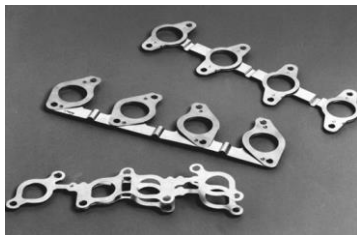
FIGURE 20-18 Typical exhaust manifold gaskets. Note how they are laminated to allow the exhaust manifold to expand and contract due to heating and cooling.
