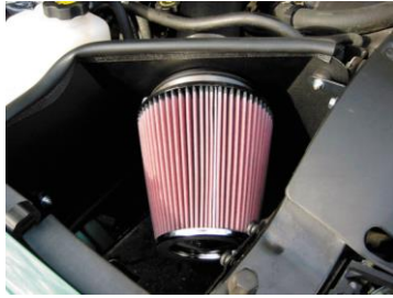
FIGURE 20–22 A high-performance aftermarket air filter often can increase airflow into the engine for more power.
