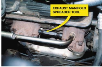
FIGURE 20-19 An exhaust manifold spreader tool is absolutely necessary when reinstalling exhaust manifolds. When they are removed from the engine, the manifolds tend to warp slightly even though the engine is allowed to cool before being removed. The spreader tool allows the technician to line up the bolt holes without harming the manifold.
