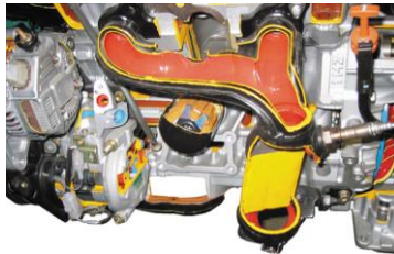
FIGURE 20–15 This exhaust manifold (red area) is equipped with a heat shield to help retain heat and reduce exhaust emissions.
