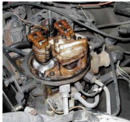
FIGURE 20-7 A throttle-body injection (TBI) unit used on a GM V-6 engine.
