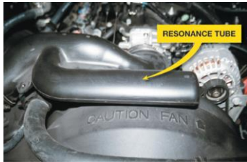
FIGURE 20-6 A resonance tube, called a Helmholtz resonator, is used on the intake duct between the air filter and the throttle body to reduce air intake noise during engine acceleration.
