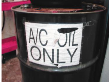
FIGURE 2-10 Air-conditioning refrigerant oil must be kept separated from other oils because it contains traces of refrigerant and must be treated as hazardous waste.
