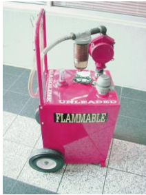
FIGURE 2-9 This red gasoline container holds about 30 gallons of gasoline and is used to fill vehicles used for training.
