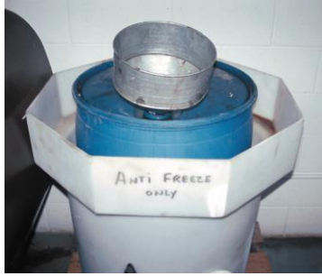
FIGURE 2-8 Used antifreeze coolant should be kept separate and stored in a leakproof container until it can be recycled or disposed of according to federal, state, and local laws. Note that the storage barrel is placed inside another container to catch any coolant that may spill out of the inside barrel.
