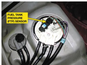
FIGURE 19–39 The fuel tank pressure sensor (black unit with three wires) looks like a MAP sensor and is usually located on top of the fuel pump module (white unit).
