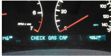
FIGURE 19–35 Some vehicles will display a message if an evaporative control system leak is detected that could be the result of a loose gas cap.
