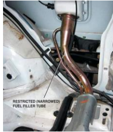
FIGURE 19-34 A restricted fuel fill pipe shown on a vehicle with the interior removed.
