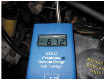
FIGURE 19-16 Using a gauge that measures vacuum in units of inches of water to test the vacuum at the dipstick tube, being sure that the PCV system is capable of drawing a vacuum on the crankcase. Note that 28 inch of water equals 1 PSI, or about 2 inch of mercury (inch Hg) of vacuum.
