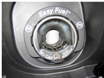
FIGURE 19–29 A capless system from a Ford Flex does not use a replaceable cap; instead, it has a spring-loaded closure.
