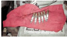
FIGURE 18–36 When removing spark plugs, it is wise to arrange them so that they can be compared and any problem can be identified with a particular cylinder.
