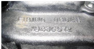
FIGURE 18–12 The firing order is cast or stamped on the intake manifold on most engines that have a distributor ignition.
