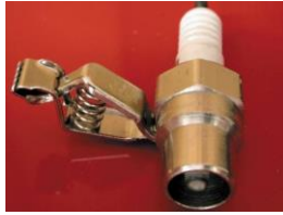
FIGURE 18–22 A spark tester looks like a regular spark plug with an alligator clip attached to the shell. This tester has a specified gap that requires at least 25,000 volts (25 kV) to fire.
