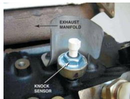
FIGURE 18–20 A typical knock sensor on the side of the block. Some are located in the "V" of a V-type engine and are not noticeable until the intake manifold has been removed.
