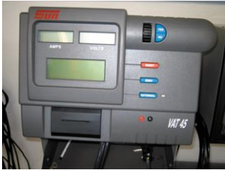
FIGURE 17-21 When connecting a starter tester such as a Sun VAT 45 to the vehicle, make certain that the inductive probe is placed over all of the cables or wires from the battery.
