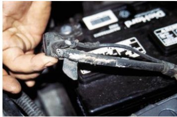
FIGURE 17-12 This battery cable was found corroded underneath. The corrosion had eaten through the insulation yet was not noticeable without careful inspection. This cable should be replaced.
