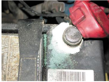
FIGURE 17-20 Carefully inspect all battery terminals for corrosion.
