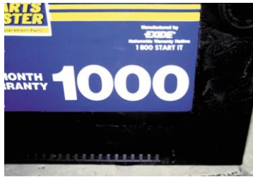
FIGURE 17-1 This battery shows a large “1000” on the front panel but this is the CA rating and not the more important CCA rating. Always compare batteries with the same rating.
