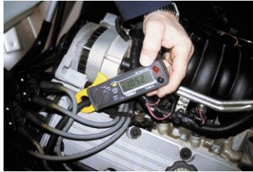
FIGURE 17-32 A mini clamp-on digital multimeter can be used to measure alternator output and unwanted AC current by switching the meter to read DC amperes.
