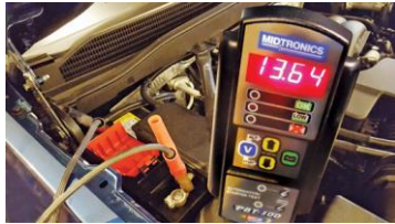
FIGURE 17-7 A Midtronics tester that can not only test the battery but can also detect faults with the starter and alternator.
