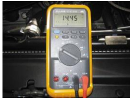
FIGURE 17-29 The digital multimeter should be set to read DC volts and the red lead connected to the battery positive (+) terminal and the black meter lead connected to the negative (-) battery terminal.
