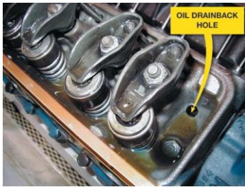
FIGURE 16–15 Oil is sent to the rocker arms on this Chevrolet V-8 engine through the hollow pushrods. The oil returns to the oil pan through the oil drainback holes in the cylinder head.
