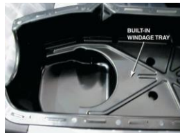
FIGURE 16–16 A typical oil pan with a built-in windage tray used to keep oil from being churned up by the rotating crankshaft.
