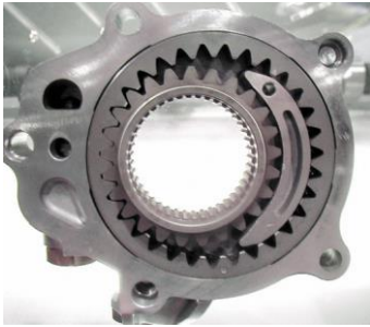
FIGURE 16-7 A typical internal/external oil pump mounted in the front cover of the engine that is driven by the crankshaft.
