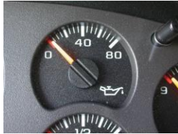
FIGURE 16-4 The dash oil pressure gauge may be a good indicator of engine oil pressure. If there is any concern about the oil pressure, always use a mechanical gauge to be sure.
