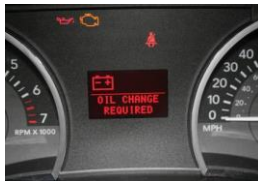
FIGURE 15-13 Many vehicle manufacturers can display the percentage of oil life remaining, whereas others simply turn on a warning lamp when it has been determined that an oil change is
