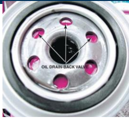
FIGURE 15-10 A rubber diaphragm acts as an antidrainback valve to keep the oil in the filter when the engine is stopped and the oil pressure drops to
