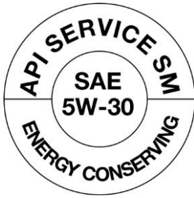
FIGURE 15–2 API doughnut for a SAE 5W-30, SM engine oil. When compared to a reference oil, the “energy conserving” designation indicates a 1.1% better fuel economy for SAE 10W-30 oils and 0.5% better fuel economy for SAE 5W-30 oils.
