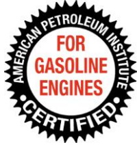
FIGURE 15-3 The International Lubricant Standardization and Approval Committee (ILSAC) starburst symbol. If this symbol is on the front of the container of oil, then it is acceptable for use in almost any gasoline engine.
