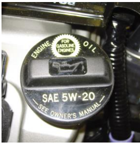
FIGURE 15-1 The SAE viscosity rating required is often printed on the engine oil filler cap. Most hybrid electric vehicles specify either SAE 0W-20 or SAE 5W-20 engine oil.
