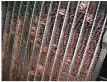
FIGURE 14-27 A heavily corroded radiator from a vehicle that was overheating. A visual inspection discovered that the corrosion had eaten away many of the cooling fins, yet did not leak. This radiator was replaced and it solved the overheating problem.
