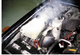
FIGURE 14-31 When an engine overheats, often the coolant overflow container boils.
