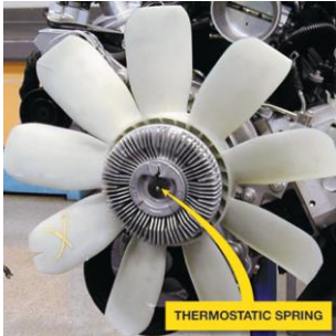
FIGURE 14-25 A typical engine-driven thermostatic spring cooling fan.
