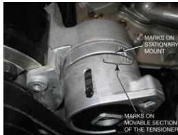
FIGURE 14-32 Typical marks on an accessory drive belt tensioner.
