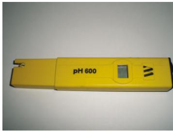
FIGURE 13-8 A meter that measures the actual pH of the coolant can be used for all coolants, unlike many test strips that cannot be used to test the pH of red or orange coolants.
