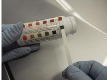
FIGURE 13–10 A test strip can be used to determine the pH and percentage of glycol of the coolant. The percentage of glycol determines the freezing and boiling temperatures, as shown on the bottle that contains the test strips.
