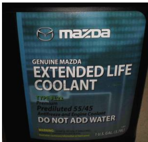
FIGURE 13-4 Coolant used in Fords that use Mazda engines and in Mazda vehicles. It requires the use of a PHOAT coolant which is dark green.
