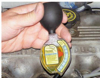
FIGURE 13-6 Checking the freezing temperature of the coolant using a hydrometer.
