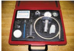
FIGURE 12-3 A gasoline testing kit, including an insulated container where water at 100°F is used to heat a container holding a small sample of gasoline. The reading on the pressure gauge is the Reid vapor pressure (RVP).
