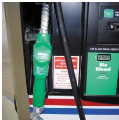
FIGURE 12-34 A biodiesel pump decal indicating that the diesel fuel is ultra-low-sulfur diesel (ULSD) and must be used in 2007 and newer diesel vehicles.
