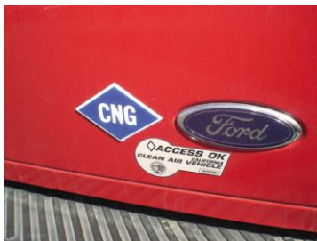
FIGURE 12-27 The blue sticker on the rear of this vehicle indicates that it is designed to use compressed natural gas. This Ford truck also has a sticker that allows it to be driven in the high occupancy vehicle (HOV) lane, even if there is just the driver, because it is a CNG vehicle.
