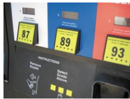
FIGURE 12-8 A pump showing regular with a pump octane of 87, plus rated at 89, and premium rated at 93. These ratings can vary with brand as well as in different parts of the country.
