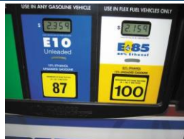
FIGURE 12-10 This fuel tank indicates that the gasoline is blended with 10% ethanol (ethyl alcohol) and can be used in any gasoline vehicle. E85 contains 85% ethanol and can only be used in vehicles specifically designed to use it.
