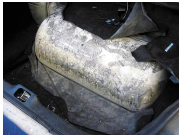
FIGURE 12-26 Propane fuel storage tank in the trunk of a Ford taxi.
