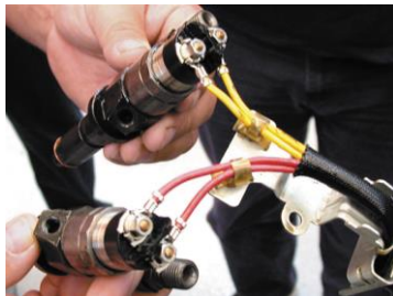
FIGURE 11-12 Typical computer-controlled diesel engine fuel injectors.
