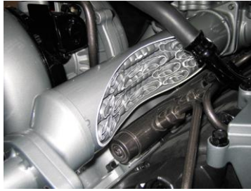
FIGURE 11-21 A cutaway showing the exhaust cooler. The cooler the exhaust is, the more effective it is in controlling NOx emissions.
