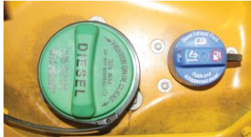
FIGURE 11–30 Diesel exhaust fluid is housed in a separate container that holds from 5 to 10 gallons, or enough to last until the next scheduled oil change in most diesel vehicles that use SCR.
