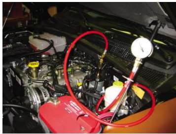
FIGURE 11-32 A pressure gauge checking the fuel pressure from the lift pump on a Cummins 6.7 liter diesel.
