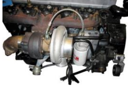
FIGURE 11-18 A Cummins diesel turbocharger is used to increase the power and torque of the engine.
