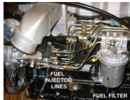
FIGURE 11-8 A typical distributor-type diesel injection pump showing the pump, lines, and fuel filter.
