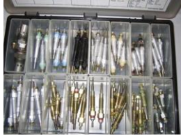
FIGURE 11–14 A glow plug assortment showing the various types and sizes of glow plugs used. Always use the specified glow plugs.
