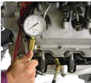
FIGURE 11-33 A compression gauge that is designed for the higher compression ratio of a diesel engine should be used when checking the compression.
