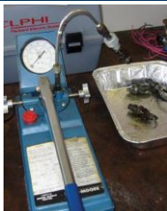
FIGURE 11-34 A typical pop tester used to check the spray pattern of a diesel engine injector.
