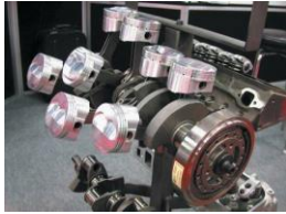
FIGURE 10-1 The rotating assembly for a V-8 engine that has eight pistons and connecting rods and one crankshaft.
