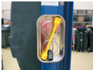
FIGURE 1-7 A magnetic tray is a helpful item to keep tools needed up where they can be easily reached without having to bend over saving time and energy over the course of a long day in the shop.
