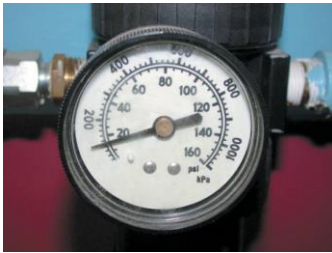
FIGURE 1-11 The air pressure going to the nozzle should be reduced to 30 PSI or less.
