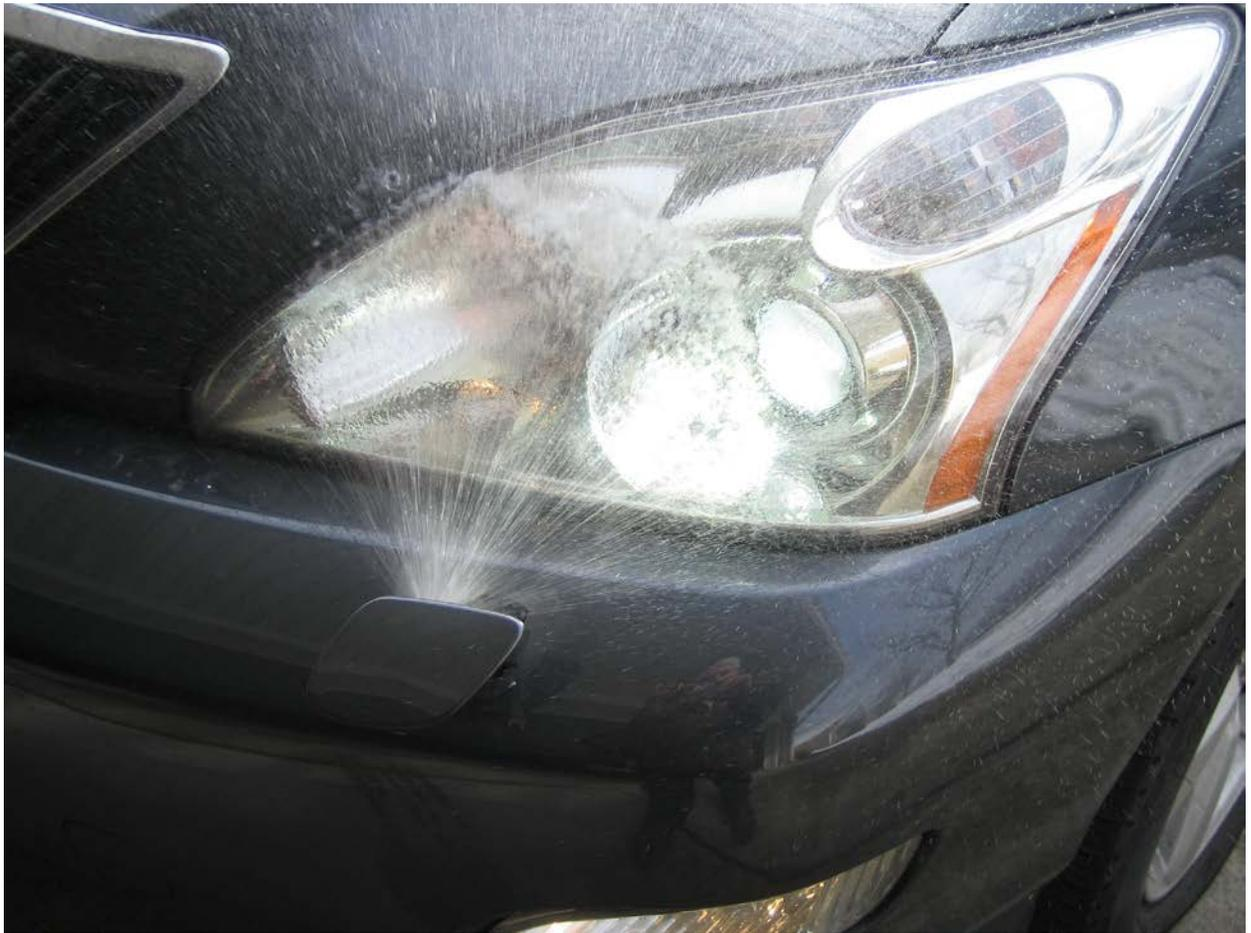
**Caption:** Headlight washers usually only work when both the headlights and the wipers are on. When the windshield washers are activated, the headlight washers spray, but usually only once per ignition key cycle.
