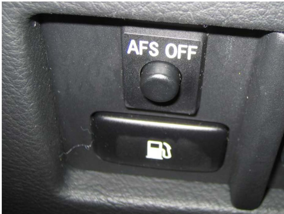
**Caption:** Typical dash-mounted switch that allows the driver to disable the front lighting system.
