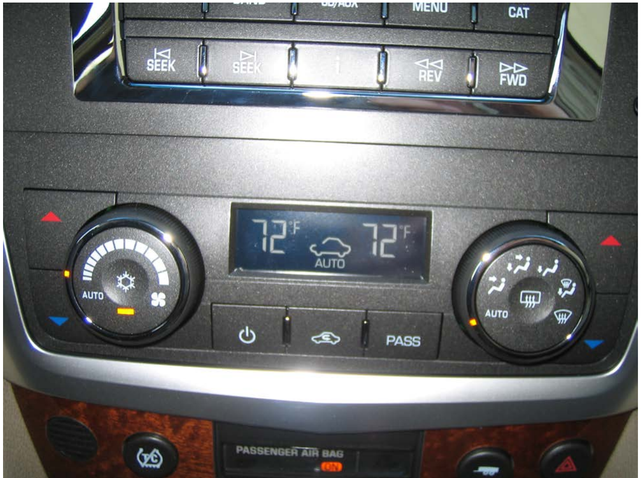
Caption: Dual-climate control panel that allows the driver and passenger to select two different temperatures.
