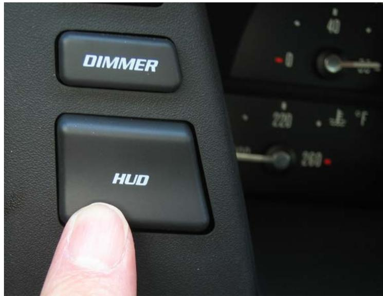
**Caption:** The dash-mounted control for the head up display on this Cadillac allows the driver to move the image up and down on the windshield for best viewing. (Photo by James Halderman)
